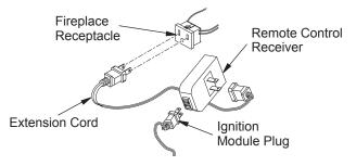
Figure 40 - Installing the WRC Remote Receiver
